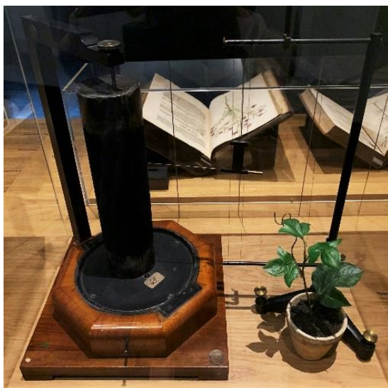
Figure 6: MAYER-SCHWIEGER also introduced the German nineteenth-century botanist Julius Sachs, who designed an instrument that measures plant movements in his pursuit of plant physiology. This auxanometer records vegetal growth in a way that has the plant itself write its record and determines the economic meaning of vegetal growth and agro-economy. © Joela Jacobs
